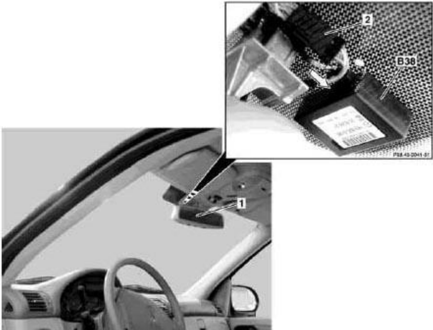
Fig. 74: Identifying Inside Rearview Mirror, Automatic Dimming Connector & Rain Sensor
